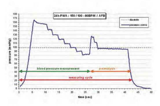
Example of a PWA. The oscillometric blood pressure measurement is combined with Pulse Wave Analysis making it very convenient for the patient
